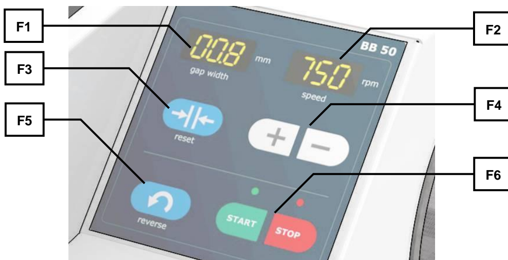
Fig. 11: View of the operator panel and displays
